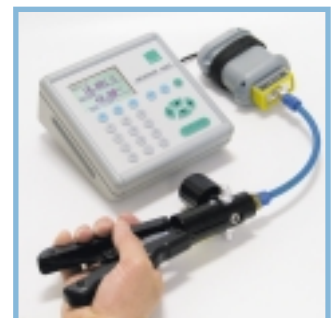
Pressure generation with hand pump
